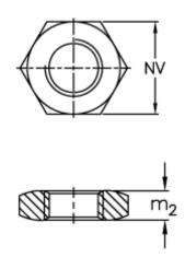
$\begin{array}{ll} m2 &= 2.7\\ Nominal size = M5\\ NV &= 8.00\\ Thread pitch = 0.80\\ Weight (g) &= 0.8 \end{array}$
